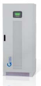
**Libra Pro** is available with a power range from 10 to 100kVA threephase/singlephase and 10 to 800kVA threephase/threephase, using double conversion on-line technology (VFI) with an inverter transformer for output galvanic isolation. The load is powered continuously by the inverter with a filtered, stabilised and regulated sinewave supply. The input and output EMI filters considerably increase the immunity of the load to mains disturbances and surges.
